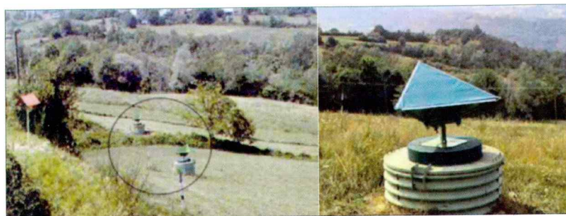
Fig. 8. Artificial rectangular permanent scatterer (TRE, 2006).
