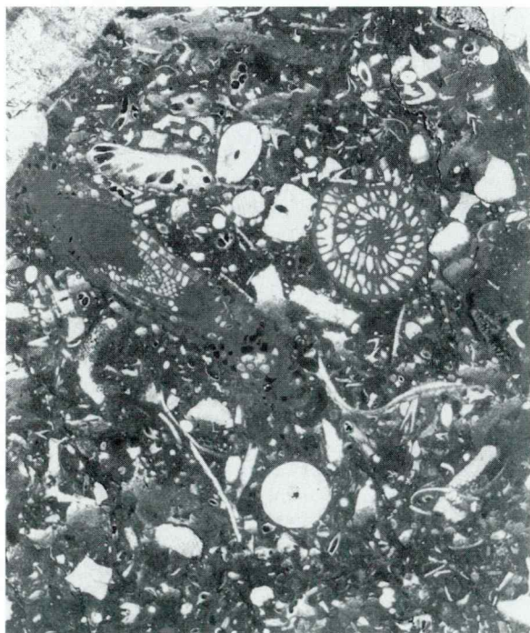
Fig. 4. Bioclastic wackestone with echinoderm fragments, fusulinids, brachiopodes and ostracods, \times 10
