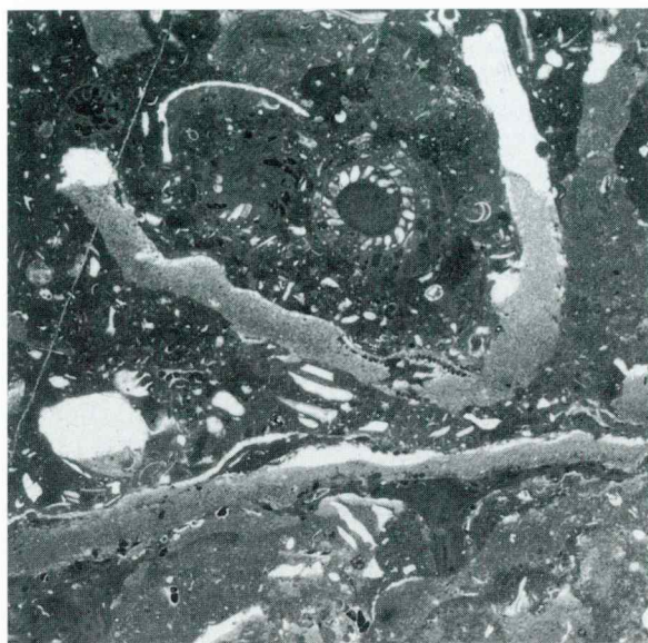
Fig. 5. Bioclastic wackestone with fusulinids, and large fragments of phylloid algae ( Eugonophyllum sp.). Internal structure mostly dissolved and filled with fine peloidal micrite, \times 10
