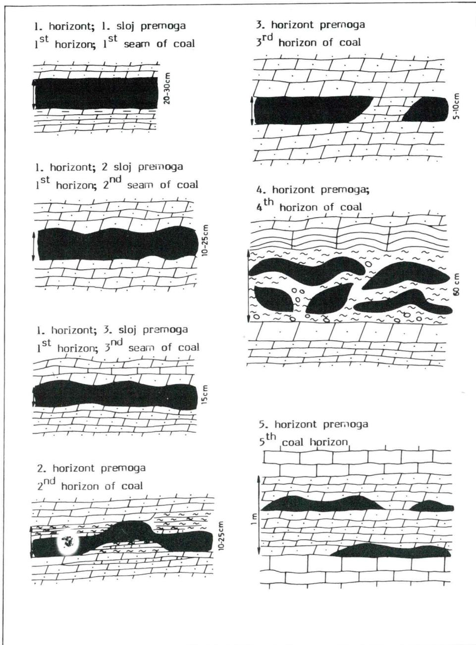
Fig. 5. Coal-bearing horizons and coal seams in the Kočevski Rog area
