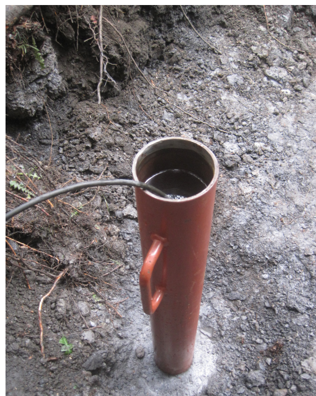
Fig. 4. Open-bottom tubes for performing falling-head test (photo: Zmag0 Bole).
