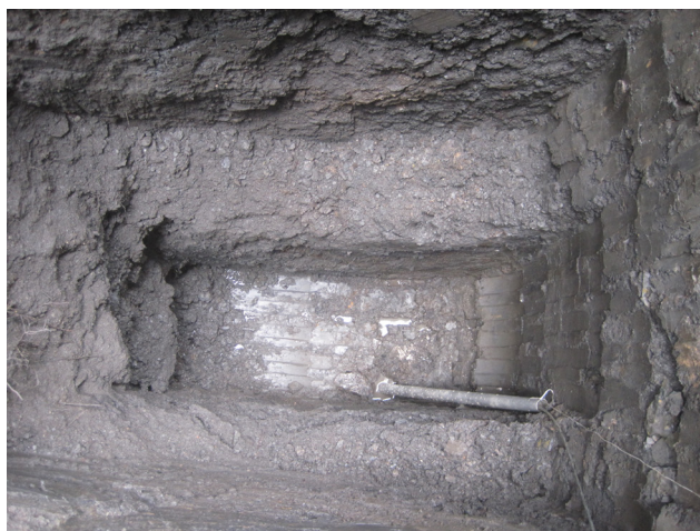
Fig. 3. Trial pit for performing falling-head test (photo: Zmag0 Bole).
