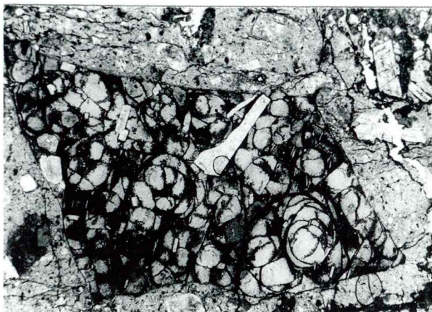
Fig. 3. Peperitic breccia; southern slopes of Krnes, near the farmhouse Atelšek. An angular clast of acid andesite composition with perlitic texture. Plane polarised light, magnification 14.5 ×
