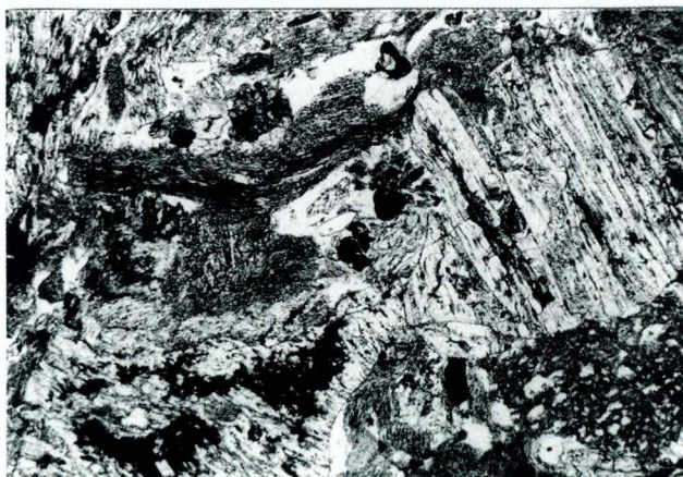
Fig. 3. Resedimented(?) pumice-rich tuff; southern slopes of Krnes. Volcanic glass of a tube pumice is replaced by heulandite, quartz and smectite. Plane polarised light, magnification 14.5 ×
