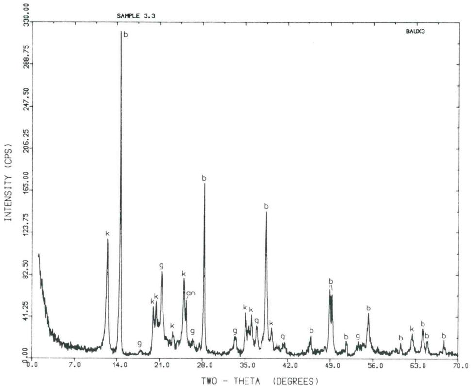
Fig. 7 XRD – diagram showing the mineralogical composition of bauxite
