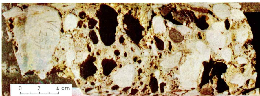
Sl. 3. Jedro poroznega konglomerata iz vrtine V-1 Fig. 3. Core sample of porous conglomerate from the borehole V-1
