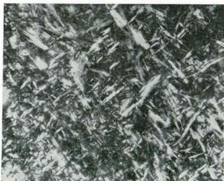
Fig. 4. Serpentinite (serpentine, talc, magnesite, accessory magnetite), \times 35 . Kajimiti bore hole I, Adola district. Determination D. Jelenc
