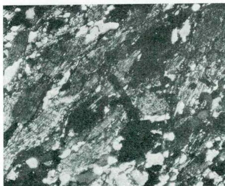
Fig. 3. Amphibolite (grains of hornblende in groundmass of silic minerals) \times 35 . Gayo Camp. Determination A. Hinterlechner
