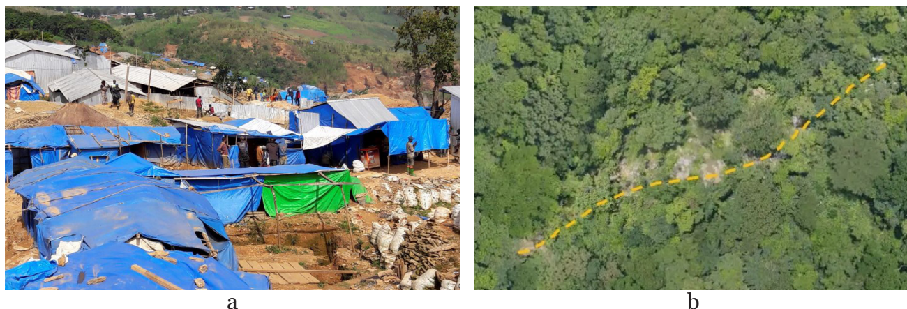
Fig. 4. Linear ASM Gold Deposits (a) A photography displaying a WNW–ESE trending ASM hardrock mining indicated by blue tarps used to cover ASM shafts, (b) Topographical image showing ASM workings along NE-SW trend (After Voormeij, 2021).
