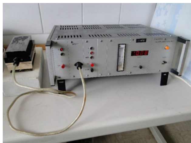
Fig. 2. Thermal conductivity meter MTP-1 (photo taken in 2022 during measurement on silicified brick).
