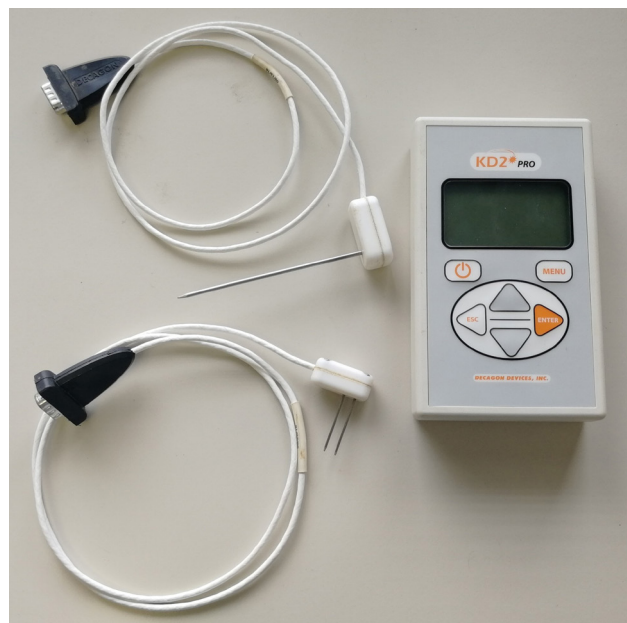
Fig. 5. The longer TR-1 single-needle probe and the shorter SH-1 dual-needle probe of the KD2 Pro Thermal Properties Analyzer.
