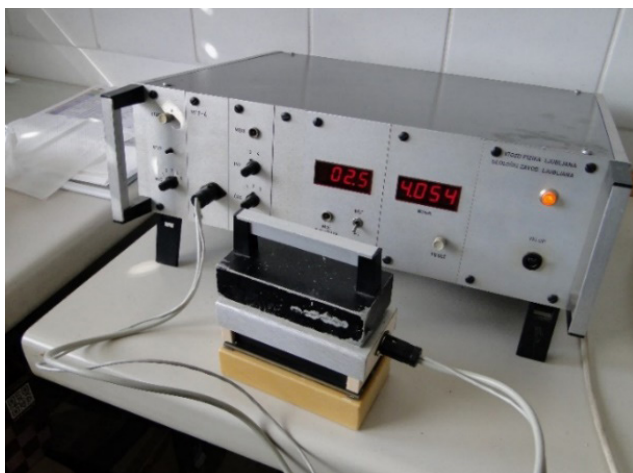
Fig. 3. Thermal conductivity meter MTP-4 (photo taken in 2022 during measurement on lacquered marble).
