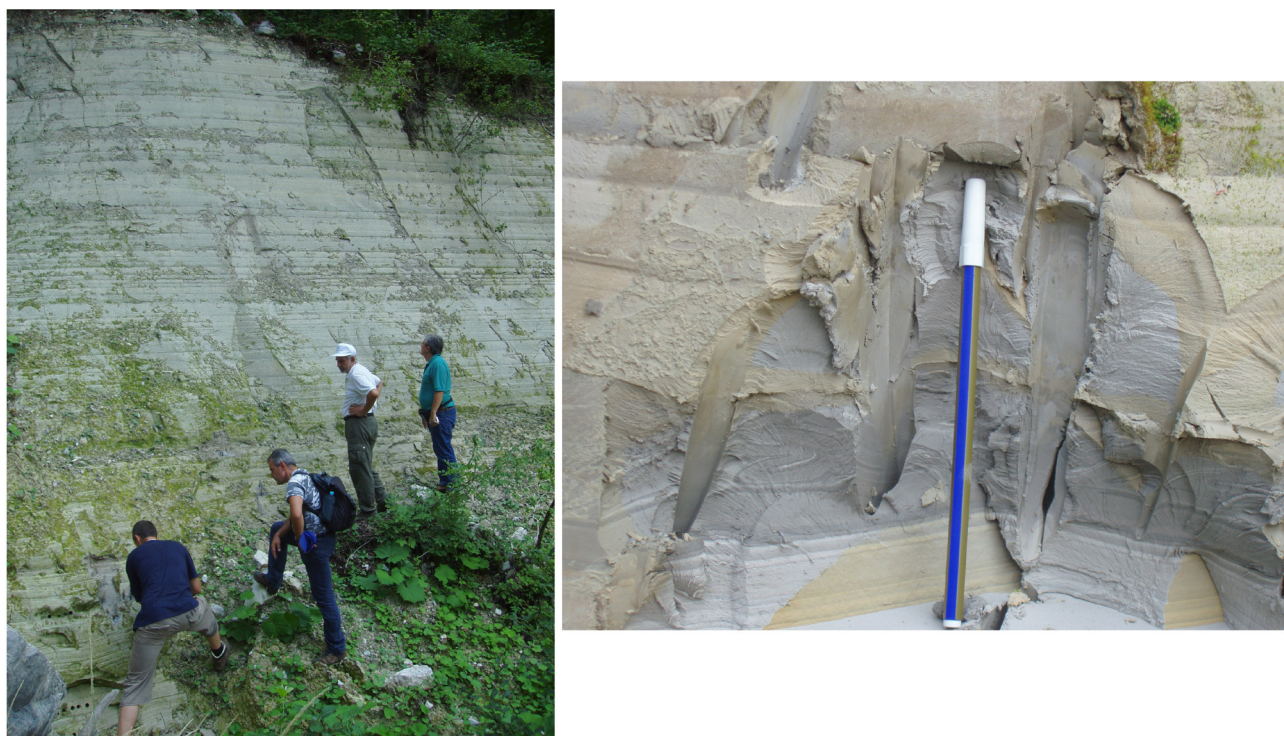
Fig. 11. Soft lacustrine sediments as exposed in abandoned clay pit near Srpenica can significantly amplify seismic ground motion and are classified as ground type E according to the Eurocode 8 standard. a) General view of thin bedded lacustrine deposits, b) close view of very soft sediment (photo: A. Gosar).
