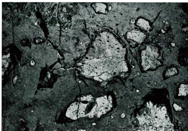
Sl. 8. Mikrosparitni apnenec z redkimi velikimi klasi. 6,5 × Fig. 8. Microsparite limestone including some larger clasts. 6.5 ×
