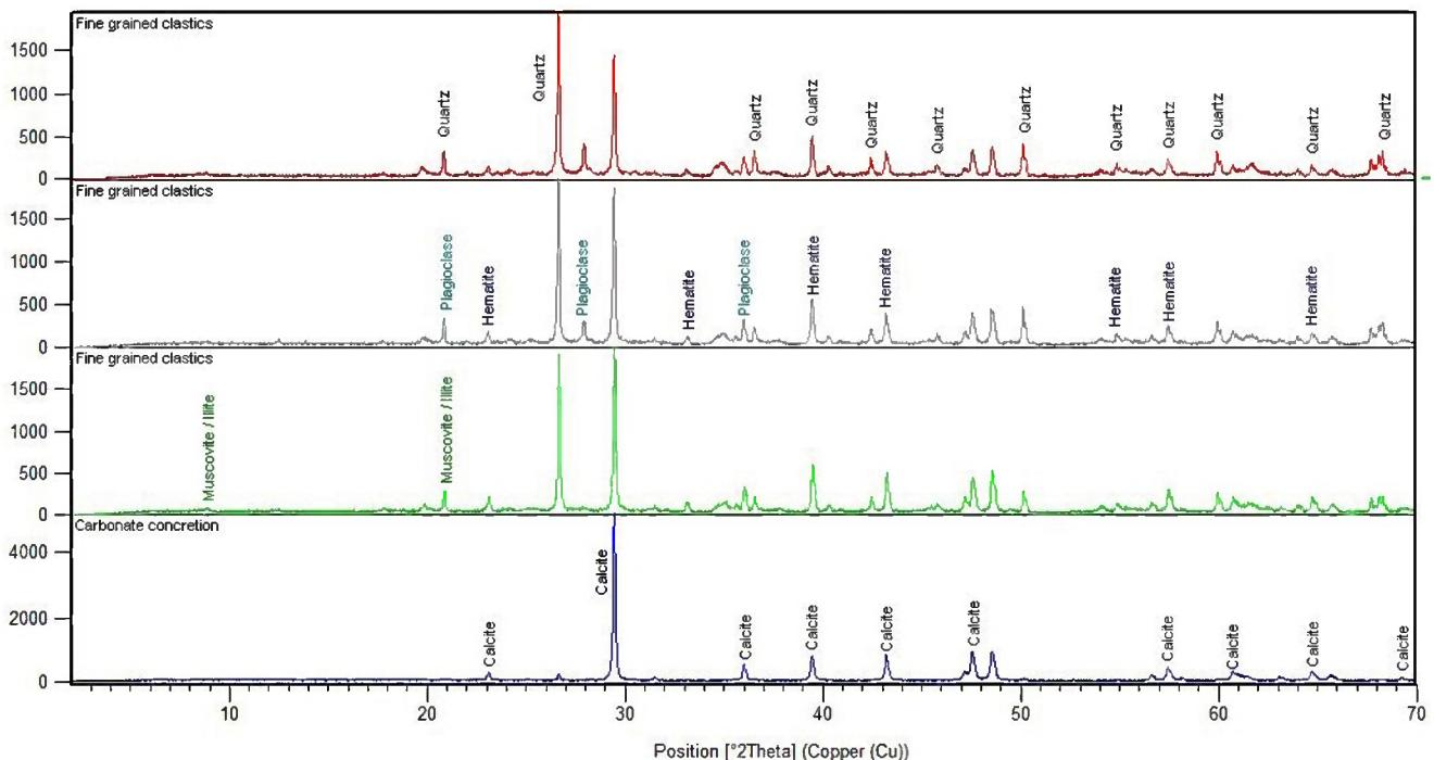
Fig. 6. Diffractograms of fine-grained clastites (upper three) and carbonate concretion (below).
