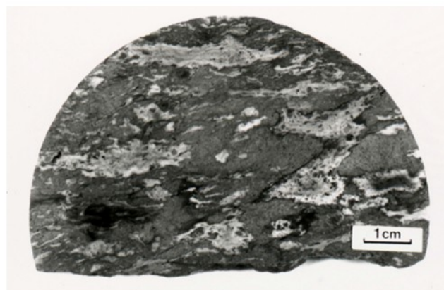
Fig. 3. Polished core surface from the borehole Tdp-1/84 at a depth of 83,2 m. Many lapilli have flame-like endings, and some of them are collapsed. Note extraordinary Z-shape above the scale
