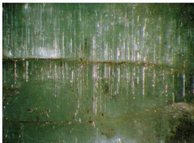
Fig. 19. Growth tube from sample V-3, 30x magnification. This type of inclusions were found in emeralds from the necklace, while those from earrings are less developed and look more like normal liquid inclusions. In emeralds from the bracelet, no such inclusions were found. Photo: Miha Jeršek
