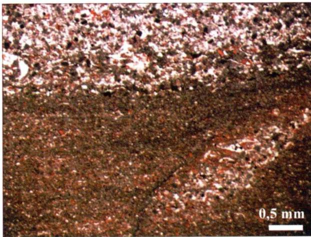
Fig. 13. Microphotograph of the sample T-18 (Streaky Limestone Member) shows a more siliciclastic bed at the top and a calcareous (micritic) bed beneath.
