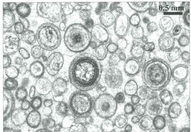
Fig. 14. Microphotograph of sample Lukač 69 shows oospiritic fabric of oolitic grainstone from the Carbonate-clastic Member. Ooids are fairly preserved and consist of core and several concentric envelopes.
