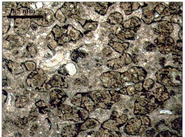
Fig. 11. Intensive dolomitisation and dedolomitisation of oolitic grainstone (Transitional Beds, microphotograph of sample Lukač G).
