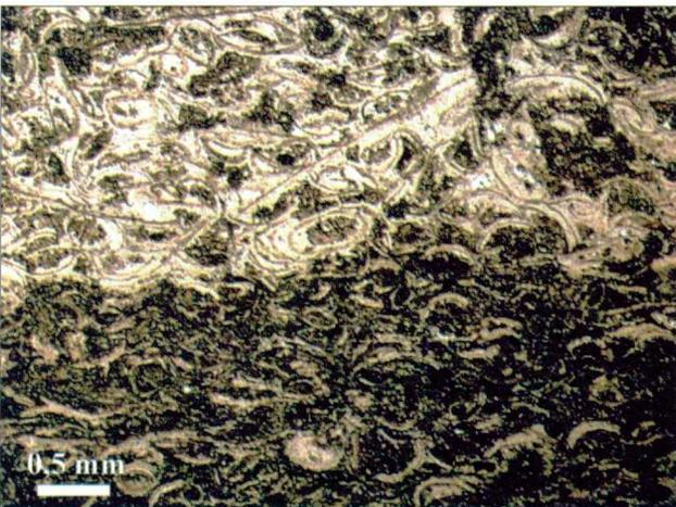
Fig. 9. The laminated micritic/biomictic limestone of the Transitional Beds is composed of dominantly micritic or dominantly bioclastic lamina. Bioclastic detritus consists often of ostracod carapaces (microphotograph of sample Lukač S).
