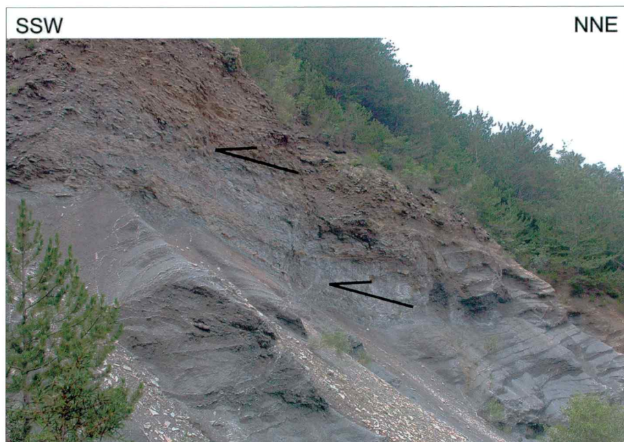
Fig. 14. Kubed Thrust Fault , diagonal transversal section of part of the fault zone. South slopes of Ivačevac hill (226m). Fault zone; in the lower part in marlstones, in the upper part in sandstones and siltstones. View from south to north.
