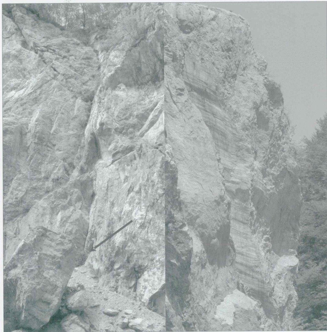
Figure 4. Left: the crack in the inner zone of the Idrija fault in the Učja valley. The arrow shows the location of TM 71 instrument. Right: The exposure of the fault plane 50 m from the crack shown in the left figure with clear striations indicating subhorizontal movements.
