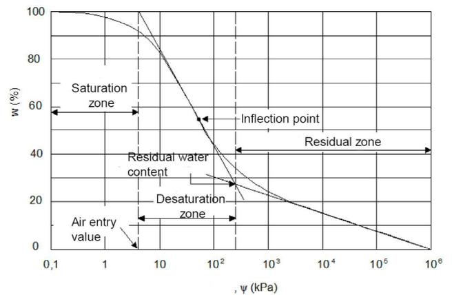
Fig. 1. A typical retention curve (SWCC: soil-water characteristic curve) (after FREDLUND et al., 2011 and KAYADELEN et al., 2007).
