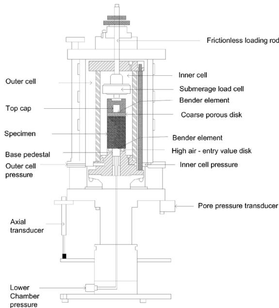
Fig. 2. The Bishop-Wesley double-walled triaxial cell.
