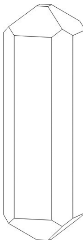
Fig. 13. Long prismatic crystal of vesuvianite from Bojtina with well-developed crystal faces of tetragonal prism of first and second order, tetragonal bipyramid of second order, and basal pinacoid.
