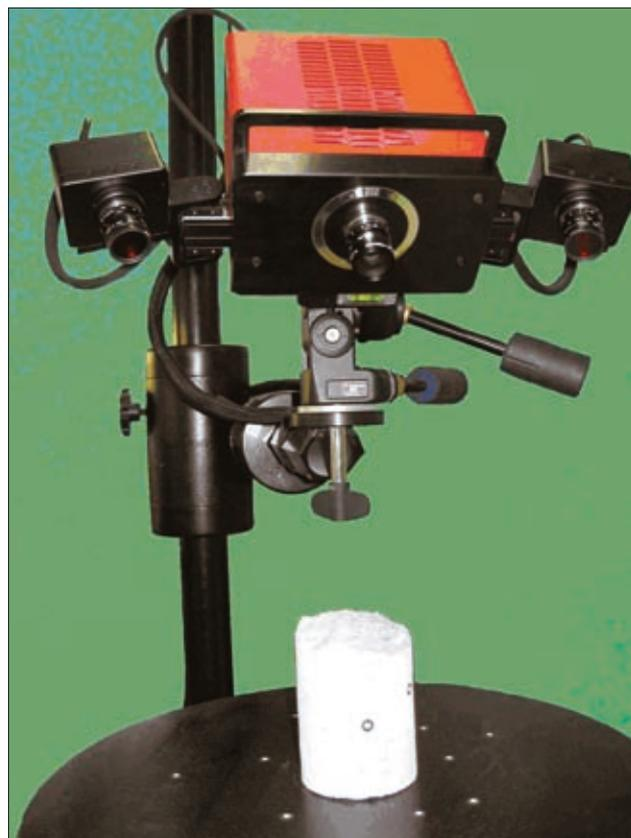
Fig. 6. The ATOS I 3D scanner and the sample
