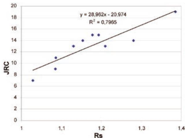
Figure 12. Comparison between the coefficients R<sub>s</sub> and JRC
